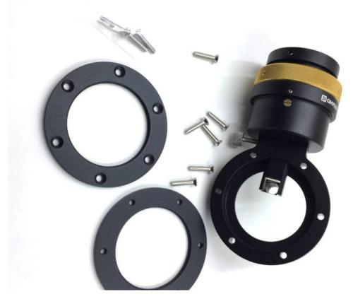
Put one piece on front of the OAG, one on back side of the OAG. Use six M3 screw to connect them. Normally speaking the one with M3 thread should be put in back side of the OAG. Now with the two piece thread adapter the total length is 16mm.
