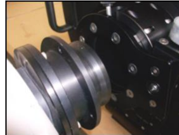
3 - Insert the 3.5" to barrel of the 200166 Reducer into the 3.5" focuser securing with the two set screws on the focuser.
