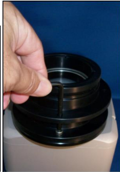
2 - Attach the 200166 Reducer to the SecureFit CCD Adapters using the four 10-32 SHC screws provided.
