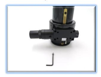
2.5mm hex key. Insert the button head screw into the countersunk hole on the motor clamp body and thread it into the threaded hole on the pinion block.
