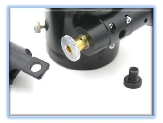
motor clamp. These are included to allow some top-to-bottom (front-to-back in relation to the telescope tube) adjustment of the motor assembly.
