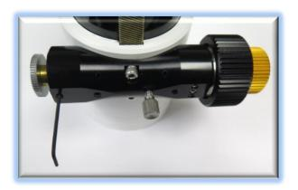
remove these setscrews, just loosen them until the coarse knob can be easily slide off the pinion shaft.
