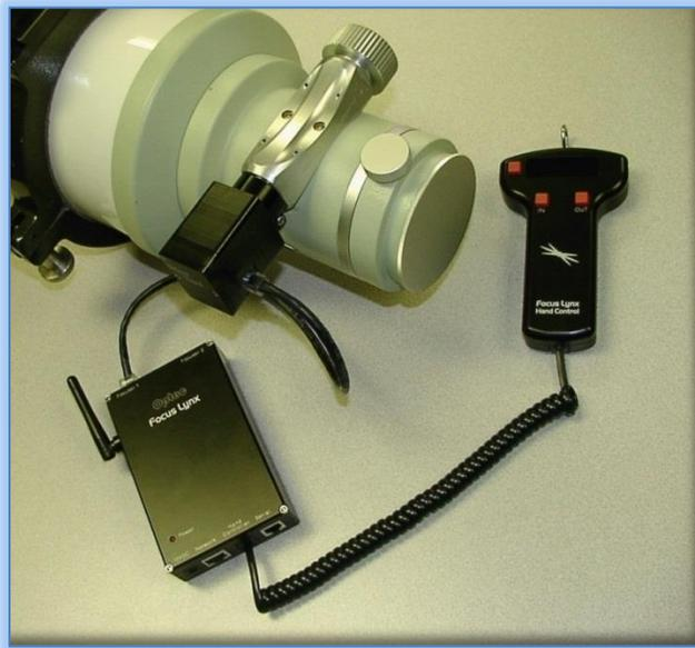
*FocusLynx Controller Hub configured for MicroTouch motor.
