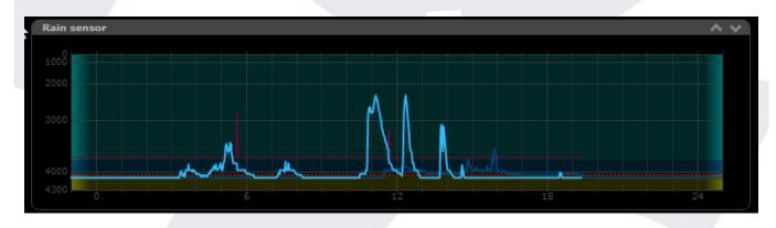
In this example can be seen the activity spikes of the heater matching the rain periods. The wind graph (and icon at the top), will show the average wind speed as a line, and the gust as a dot:
