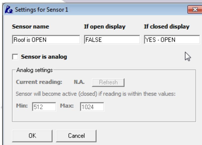
for the roof (roll off roof) we suggest using two switches, one for signaling “open” and other to signal “closed”, this way we will notice should the roof stop mid-travel.
