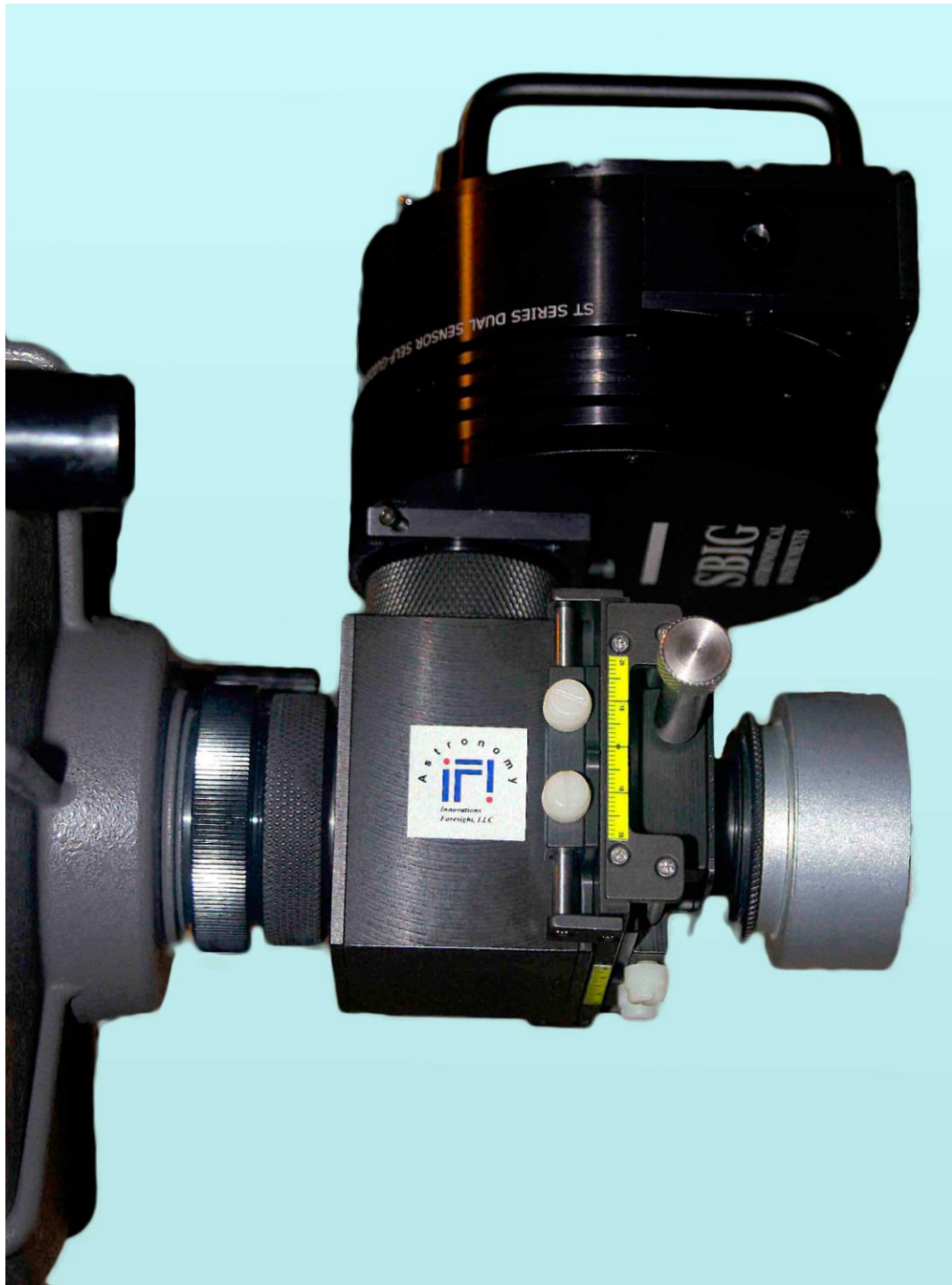
ONAG® mounted on Celestron 8" ("orange" tube) with SBIG ST2000XCM imager and Orion StarShoot autoguide
