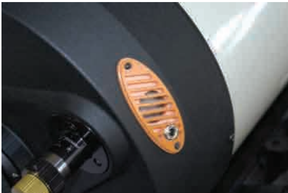
Image 1 – Celestron EdgeHD optical tube showing TEMP-est rear-collar fans (available in multiple colors, including black).
