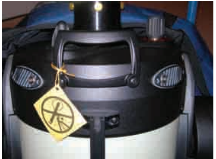
Image 3 – Rear TEMP-est fans in black, mounted on a Celestron CPC Deluxe 1100-HD
