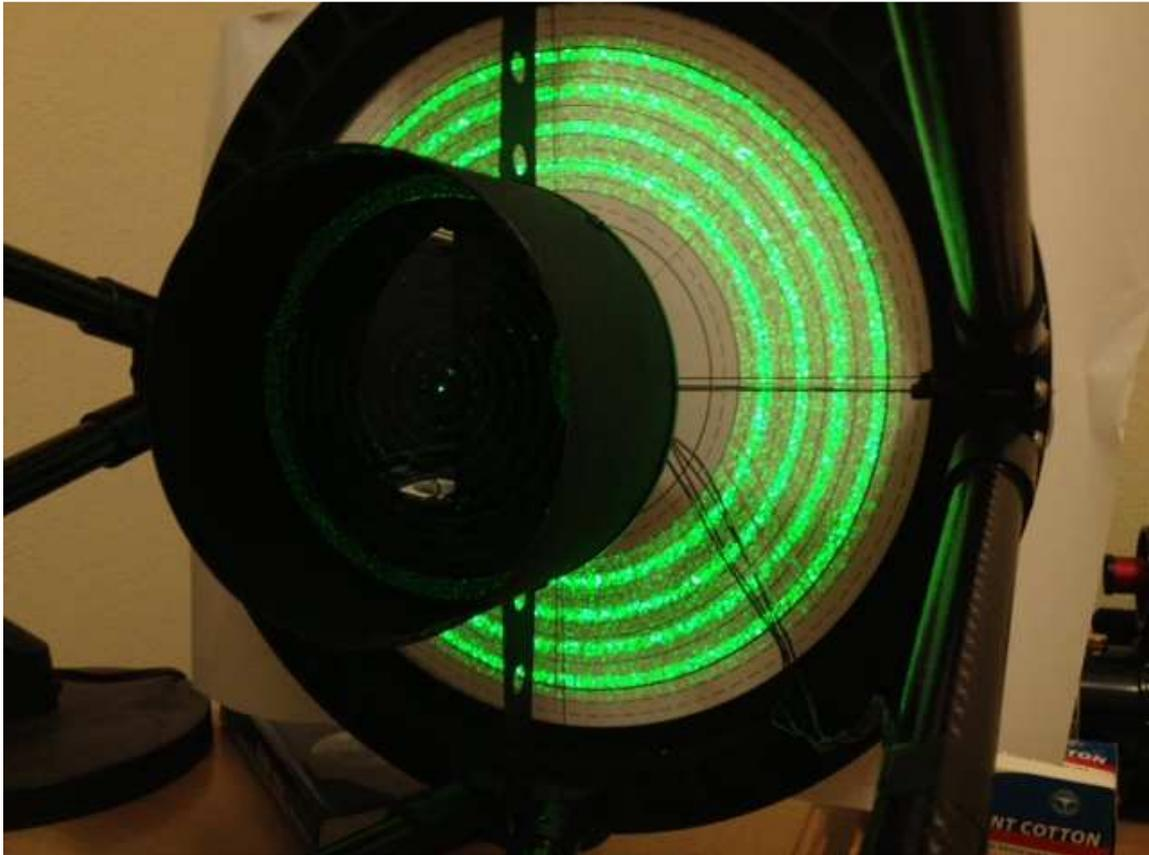
Figure 3 Laser ring projection pattern on front aperture of a 12.5" iDK telescope (Image courtesy of Tim Khan)
