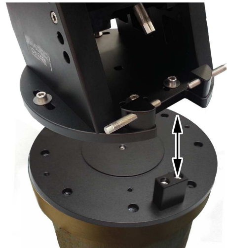
Fig. 4.10: Mount and base adapter alignment.
