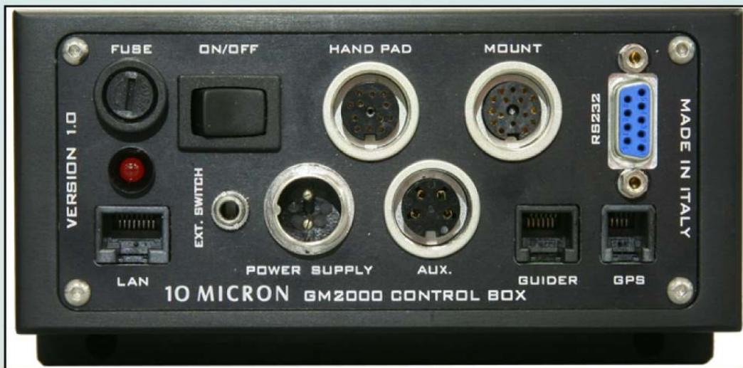
*The connections of the control box.*
