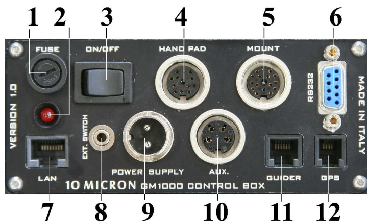
Fig. 5.1: The connection panel on the control box.
