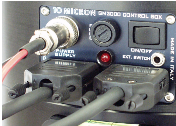
Fig. 5.12: Motor cables and power supply connections.
