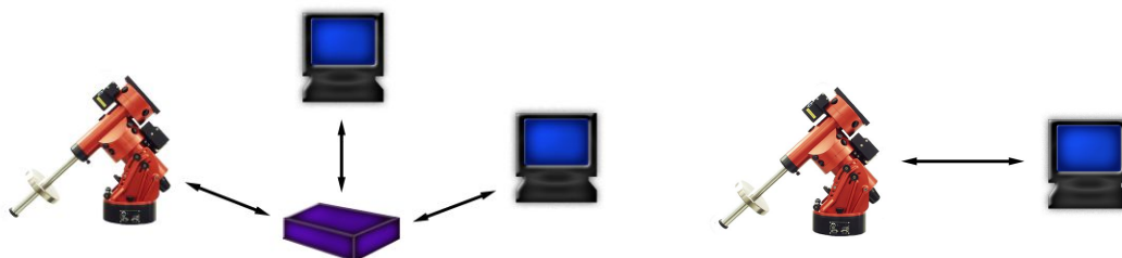
Fig. 9.1: Connecting the mount to a network. Fig. 9.2: Connecting the mount directly to a PC.
