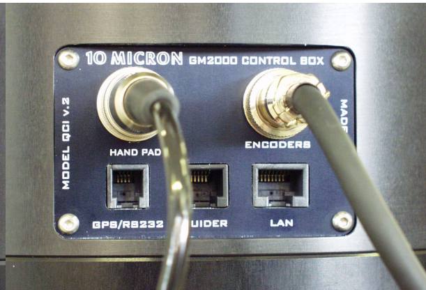
Fig. 5.13: Encoders cable and hand pad connections.
