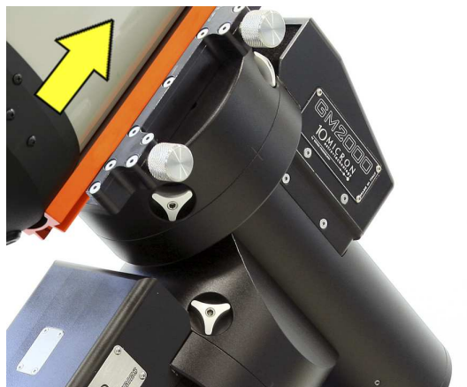
Fig. 4.16: This is the position to attach the counterweights and the telescope.
