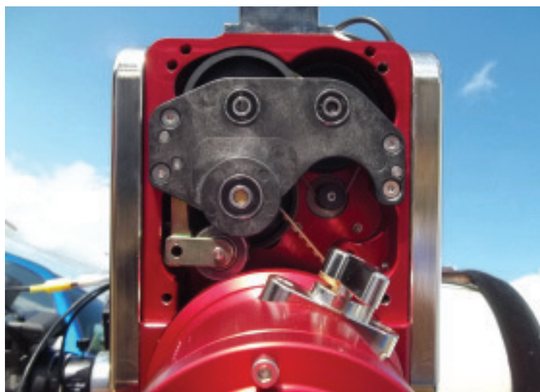
Image 4 - The M-Uno's "Fast Reverse" drive: a tooth belt-pulley system.
