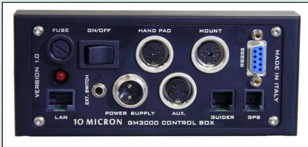
The control box on the GM3000HPS.
