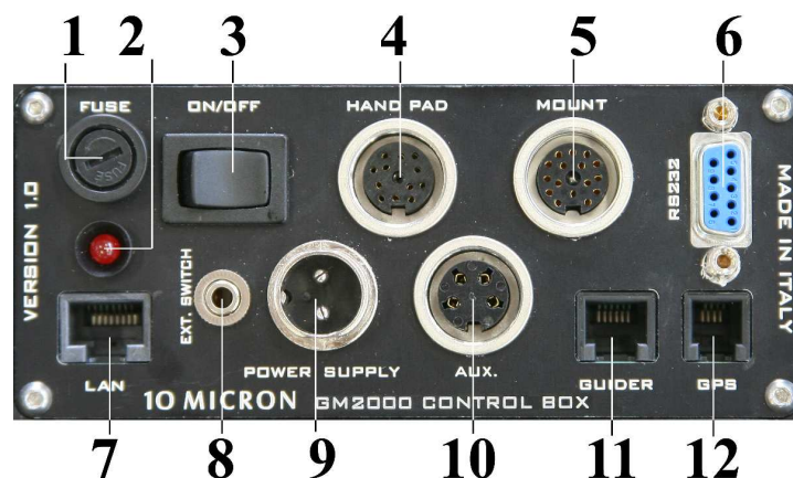
Fig. 5.1: The connection panel on the control box.
