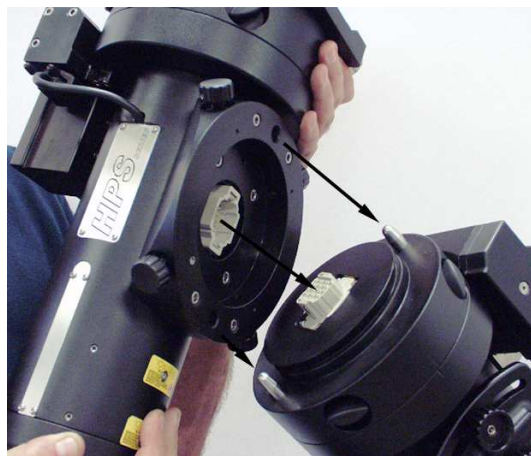
Fig. 4.15: Ultraportable version assembly.
