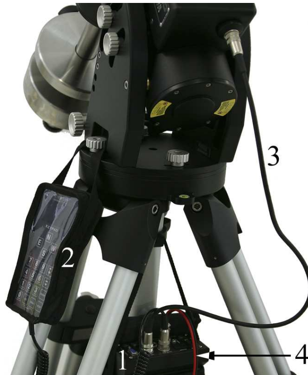
Fig. 5.7: Electrical setup. 1 – control box; 2 – keypad; 3 – mount cable; 4 – power supply cable.
